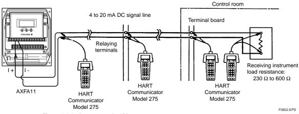
Figure 8.1.1 Interconnection Diagram
